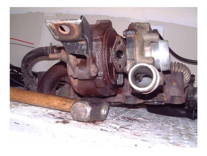
DO NOT hit the ALUMINUM!!! Verify with every hit you are on the cast iron bearing housing!!!
